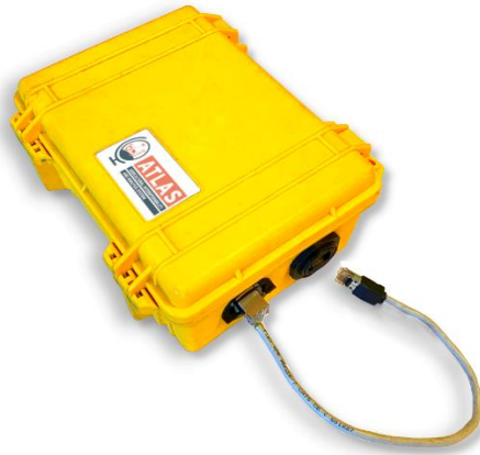
Figure 2: edge computing system in a protective casing to be installed in the barn.
